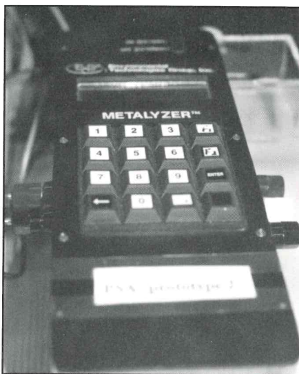
Dr. Joseph Wang has developed a "lab-on-a-chip," a control unit including a compact, battery-operated analyzer that can record data and operate unattended. (Photo by Alison Sawyer)
