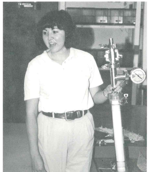
Biology graduate student Linda Winona describes the operation of a hollow-fiber ultrafiltration system to be used to concentrate viruses from large volumes of river water.
